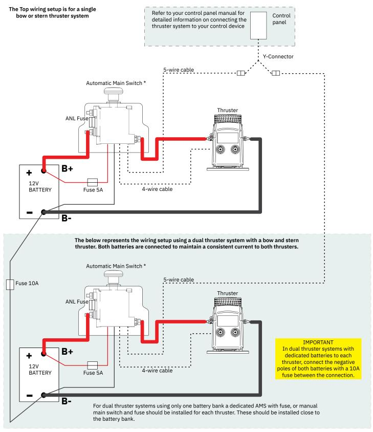
\*Automatic Main Switch can be replaced by a fuse holder and manual main switch.
