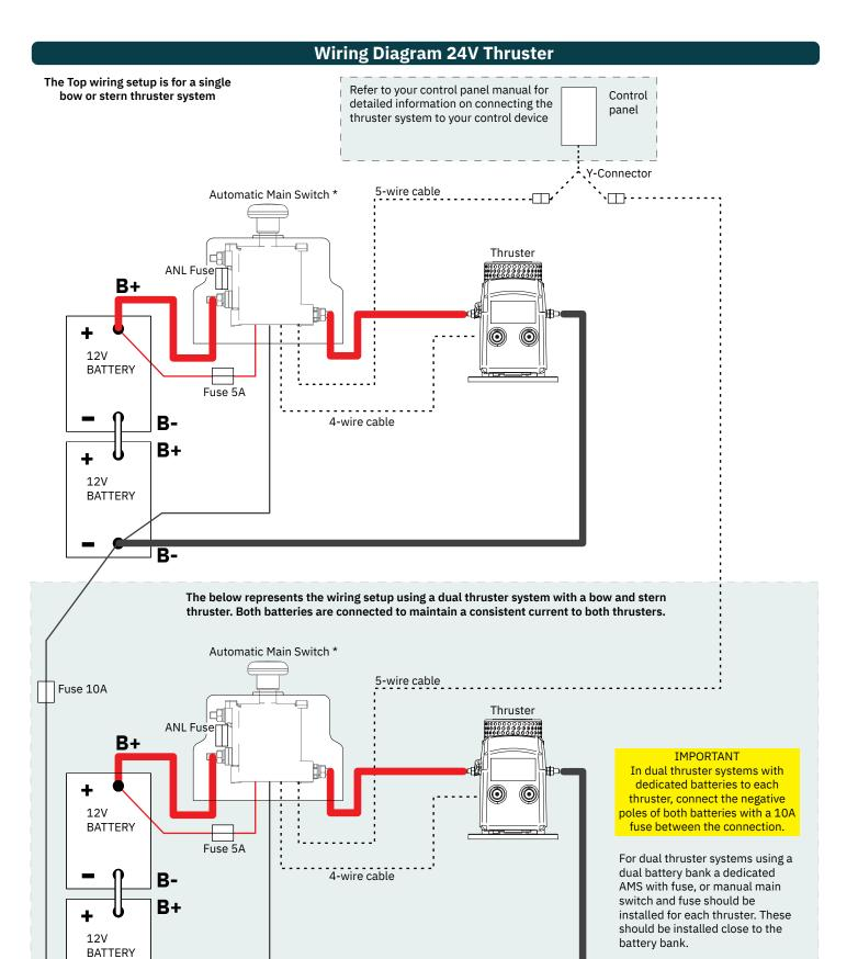
\*Automatic Main Switch can be replaced by a fuse holder and manual main switch.
